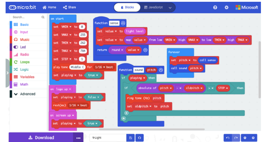
Figure 7: The 'sound' function prevents clicky sounds. Detecting a change in a value, is a common programming pattern.
